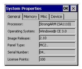
The «General» tab contains important information about the device and the installed Windows CE version. «Image Release» shows the version of the CE Image. See also the chapter <u>Licensing</u>.
